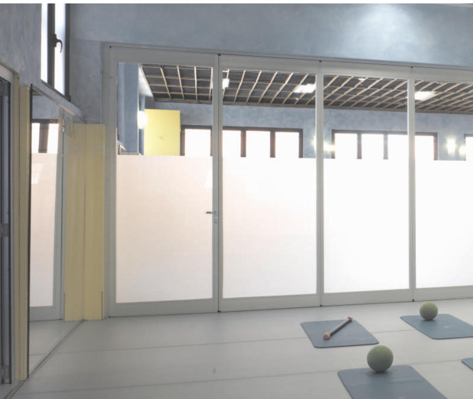
*Domino is the operable partition composed by independent modular elements that, when closed, makes a continuous partition perfectly aligned. The elements slide by ball bearing trolleys in a track fixed to the ceiling.*
